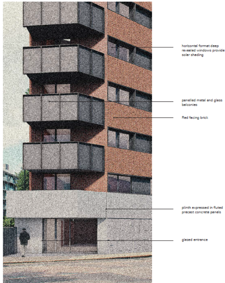
Southern Elevation - Detail Study
